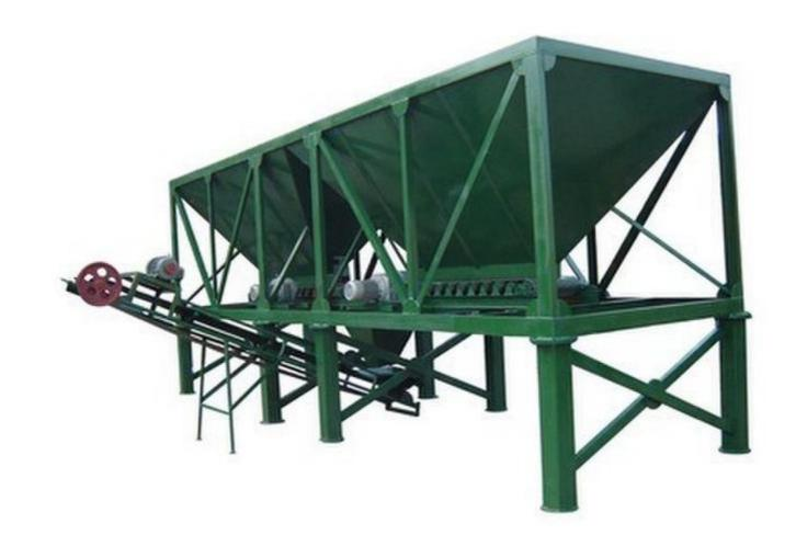
Hammer mill system: In order to ensure that the size of biomass material entering the furnace is less than 3mm, rice husk and crushed corncob need to be crushed for the second time, the system is designed with a set of hammer mill, the feeding size of the hammer mill shall not be greater than 80mm, the discharging size shall be less than 3mm, and the system output shall be 10-15 t/H.
